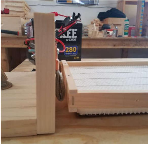
Press frame into embedder contacts.
