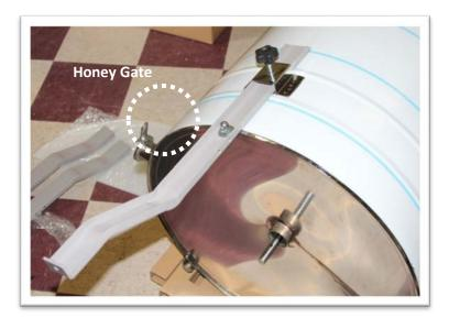
3. Bolt on the legs. You will need a large washer, small washer, cap nut, and bolt for each leg (see inset below). Place the small washer in between the leg and the extractor. Place the large washer between the nut and the outside of the leg. After installing the bolts, install the hand knobs to clamp the legs in place.
