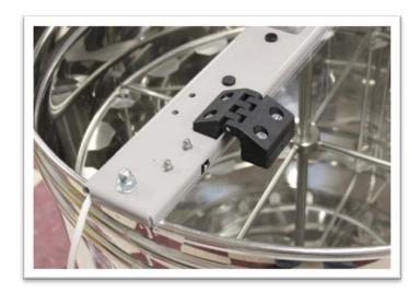
15. Install the motor controller on the top bar. You will need to remove the two small plastic plugs from the top bar. The digital screen will face you on the left side of the extractor. See below for orientation.
