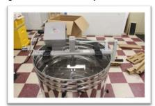
16. Connect the motor cable and mount the connector on the leg with two zip ties as shown.
