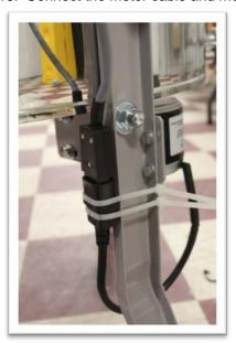
17. Route the motor wire as shown and mount on the extractor drum with adhesive mounts and zip ties. Place the adhesive mounts in the locations shown by arrows, below.
