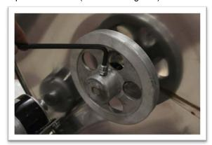
8. After hex cap screw is tightened, lock it in place by tightening the nut onto the pulley with an open end wrench.
