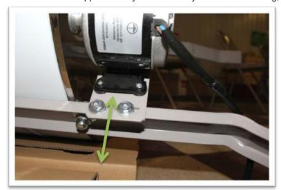
10. Install the belt on the motor pulley, and force the belt onto the large pulley by rotating the large pulley by hand. There should be no slack in the belt once installed. If there is, remove belt, slide motor outward, and reinstall belt.
