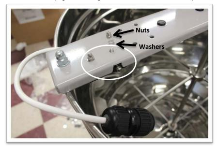
12. Loosen the top bar nut on the lid switch side (but do not remove), lift the bar  $\sim 1/8$ ", and slide the lid switch cord underneath the top bar. Re-tighten the nut.
