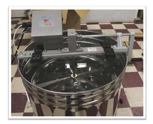
21. Clean extractor before use. **Be sure to unplug the extractor first and do not get the electronic components wet.** Regular dish soap and warm water is sufficient.
