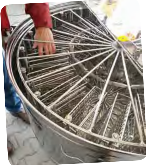
A cassette extractor. Not common in the US, but an option for places that extract extremely thick honey. Available by special order.
