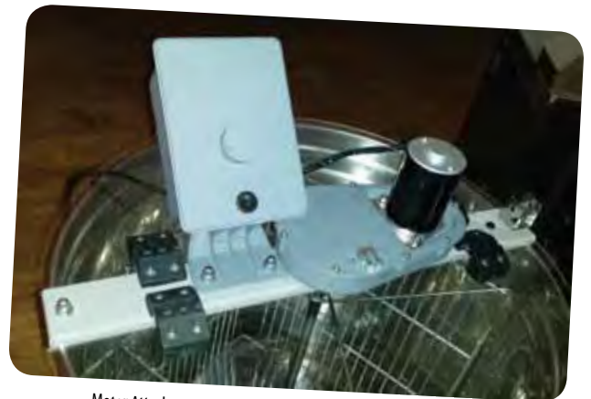
Motor Attachment that will be available for smaller hand crank units. This unit is still in the development stages, but will provide an affordable way to upgrade your manual extractor to a motorized extractor. Stay tuned!
